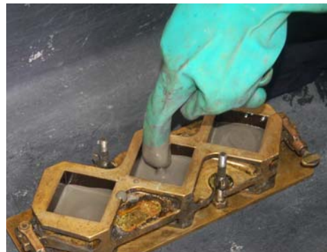
Puddle 5 times with gloved finger or tamping rod.
