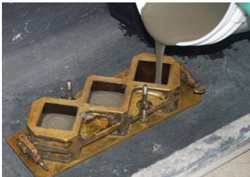
Fill cube mold ½ way with fluid/flowable grout.
