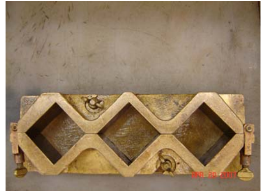
2" x 2" brass cube mold with cover plate
