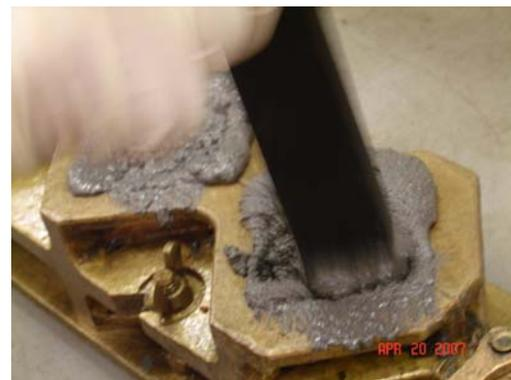
Fill molds halfway with epoxy grout then tamp or rod to remove entrapped air.
