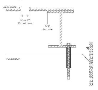
D. When grouting skid mounted equipment or frames, provide a four to six inch diameter (100 to 150 mm) grout filling hole in the center of each bulkhead section.
