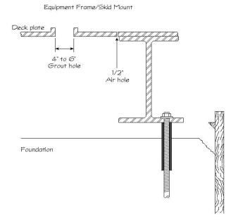
D. When grouting skid mounted equipment or frames, provide a four to six inch diameter (100 to 150 mm) grout filling hole in the center of each bulkhead section.
