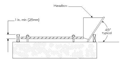
C. Height of formwork shall extend a minimum of one inch (25 mm) above bottom edge of the baseplate. Grout forms shall have one inch (25 mm) chamfer strips at all vertical corners and top edges of grout shoulders.
