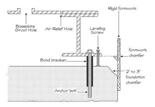
D. All formwork shall be coated with a bond breaker such as two coats of paste wax or polyethylene. Form release oil is not acceptable. Caution: Care should be taken not to contaminate grouting surfaces where bond is required.
