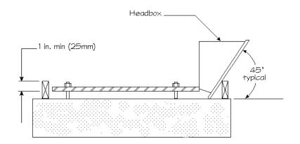
C. Height of formwork shall extend a minimum of one inch (25 mm) above bottom edge of the baseplate. Grout forms shall have one inch (25 mm) chamfer strips at all vertical corners and top edges of grout shoulders.
