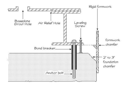
D. All formwork shall be coated with a bond breaker such as two coats of paste wax or polyethylene. Form release oil is not acceptable. Caution: Care should be taken not to contaminate grouting surfaces where bond is required.
