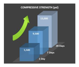
Non-shrink from time of placement, High Strength 130 Grout is easy to place and can be installed at temperatures between 40°F and 90°F (4°C and 32°C).
