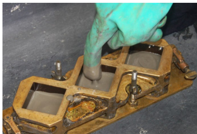
D.2. Puddle 5 times with gloved finger or tamping rod.
