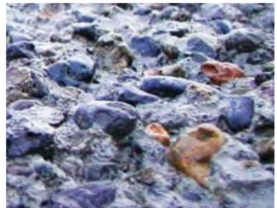
CSP10 - SURFACE PREPARED USING HIGH-PRESSURE WATER JETTING.
