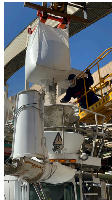
DISCHARGING BULK BAG CONTENTS INTO TRUCK INLET
