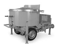
For mini bulk bag mixing and pumping applications, Five Star Products does allow the use of a vertical shaft mortar mixer with the following caveat: \*Because of the limited shearing action of a vertical shaft mixer, more water may be required to completely mix Five Star® cementitious products. The addition of more water may result in lower than published compressive strengths.
